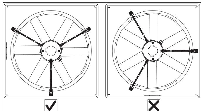
Illustration 3: Condensate drain hole at lowest possible position
