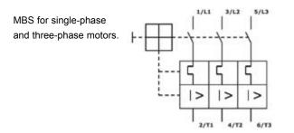
MBS reacts to the thermocontact for single-phase motors (MBSESC10ZK).
